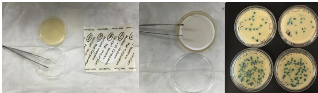
Figure 15-MI agar medium and the filter (left). Filter placed on the plate (Middle), MI agar plates after incubations (right)
